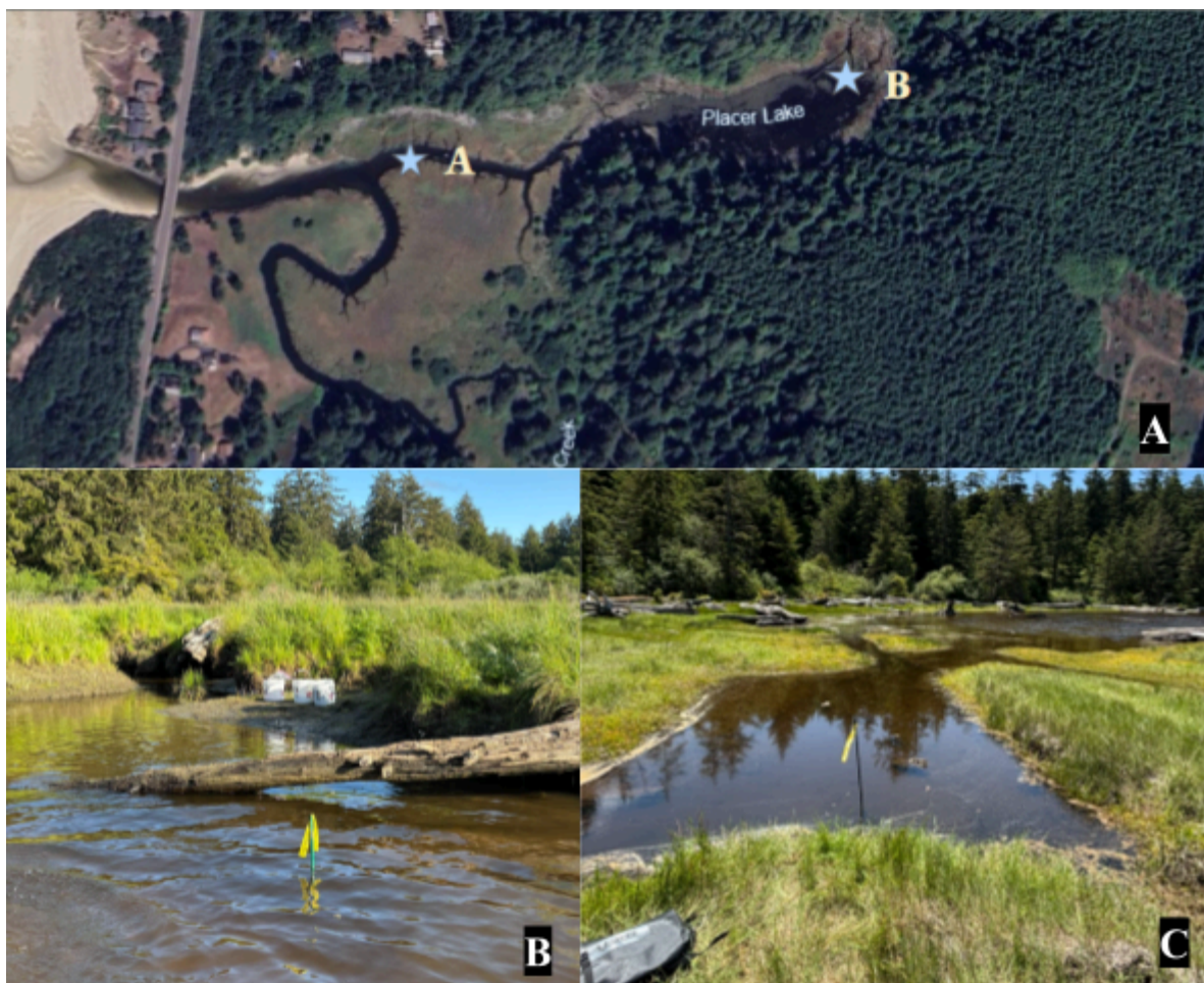
Fig 5. Hobo Conductivity Logger location in the Placer Lake and Reynolds Creek water system (a), with Logger A (b) placed in the main channel and Logger B (c) at the eastern most end of the lake. Blue stars represent their geographic location in the waterbody (a) and their unique ID is represented in the adjacent yellow letters A and B.
